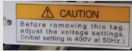
Compressor warning label
