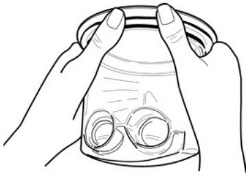
Removing the chamber base
